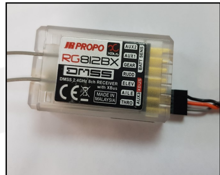
Please note cable polarity on a RG812BX
