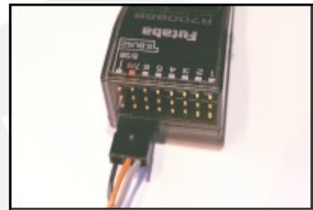
Please note cable position on a 7008 receiver. It is possible to plug into the ground pins of the receiver and this may damage the receiver and Smooth Flite system.
