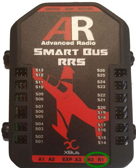
Ensure that the RRS cables supplied is plugged into the R2 and R1 port of the Smart Bus
