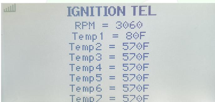
The text based telemetry has been calculated by the AR engineers to show in degrees F. It shows RPM and temperature for up to 7 cylinders. If temperature slots are not populated then the temperature value shows NC (not connected). Maximum temperature for display is 570F (300C)
