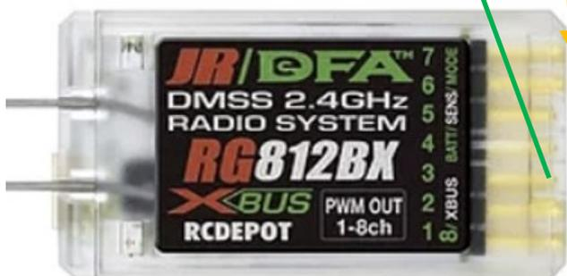
Connect from your chosen receiver Ignition Switch Channel to ARBUS Input using supplied AR1 to JR lead. This will be the IGNITION KILL SWITCH channel
