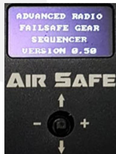
**WARNING**—Air Safe will power air valves, servos (for gear doors) and linear actuated electric retracts i.e. retracts that connect with a servo lead. It is not designed to directly power electric DC motor retracts.
